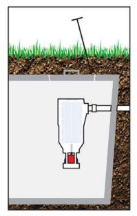
Locate the outlet of the septic tank.
