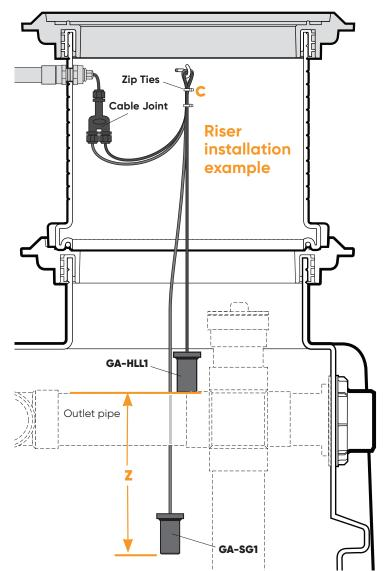
**5.** Attach sensor cables to Cable Joint as described in manufacturers manual.
